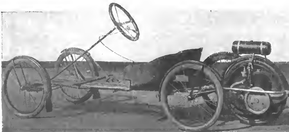
Smith Flyer two-passenger four-wheel buckboard driven by Smith motor wheel
